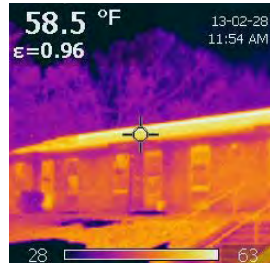
An infra-red image of one of the buildings. The brighter colors indicate warmer surfaces, possible heat loss. Roof surface is heat gain from sunlight.
